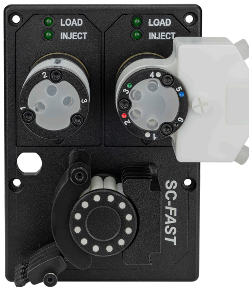
Figure 1. Integrated DXi valve assembly for SampleSense Clinical for NexION 2000.
